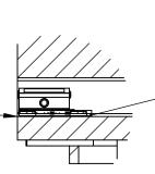
Packing may be required so slide system can protrude past boot door / opening
