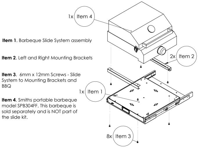
NOTE, THE 8MM BOLTS, NUTS AND WASHERS (MINIMUM 4 TO BE USED) ARE NOT SUPPLIED AND TO BE SUPPLIED BY THE INSTALLER. THESE ARE USED TO SECURE THE SLIDE SYSTEM TO THE CARAVAN, RV OR CAMPER TRAILER. THESE MAY BE DIFFERENT DEPENDING ON THE MAKE AND MODEL OF THE CARAVAN, RV OR CAMPER TRAILER.
