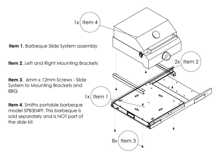
NOTE, THE 8MM BOLTS, NUTS AND WASHERS (MINIMUM 4 TO BE USED) ARE NOT SUPPLIED AND TO BE SUPPLIED BY THE INSTALLER. THESE ARE USED TO SECURE THE SLIDE SYSTEM TO THE CARAVAN, RV OR CAMPER TRAILER. THESE MAY BE DIFFERENT DEPENDING ON THE MAKE AND MODEL OF THE CARAVAN, RV OR CAMPER TRAILER.
