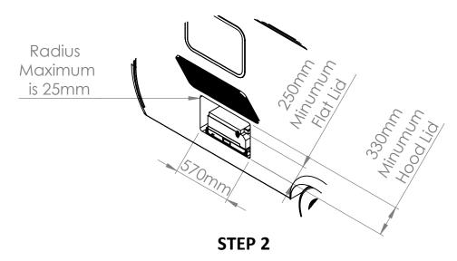
The Smiths Slide System is designed to be installed flush with the bottom of the tunnel boot opening. If the floor is lower than this opening, packing such as melamine/mdf/ply will be required to be placed between the floor and the slide system to raise the slide system to the correct height.
