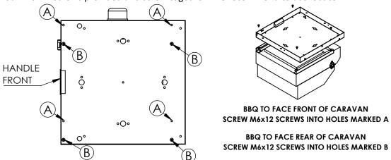
The gas connection must be carried out by an authorised and licensed gas fitter and the installation must meet the Australian and New Zealand Standards AS/NZS5601 and AS/NZS5263. See Smiths Barbeque user manual and install instruction.
