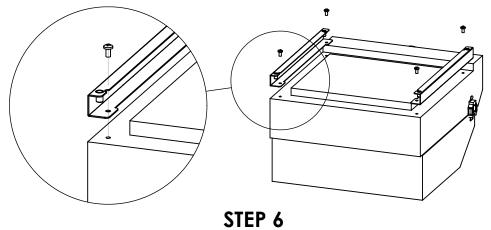
Unclip the bbq slide system and pull it out to it's fullest extension. Position the barbeque onto the slide system so that the barbeque sides are parallel with the caravan side. You must not fit the barbeque so the front of the barbeque is parallel to the caravan side as the hood will hit on the caravan side. If you want to mount the barbeque so the front is parallel with the caravan side, you must install the Smiths Slide System SBBQS800 - 800mm model.
